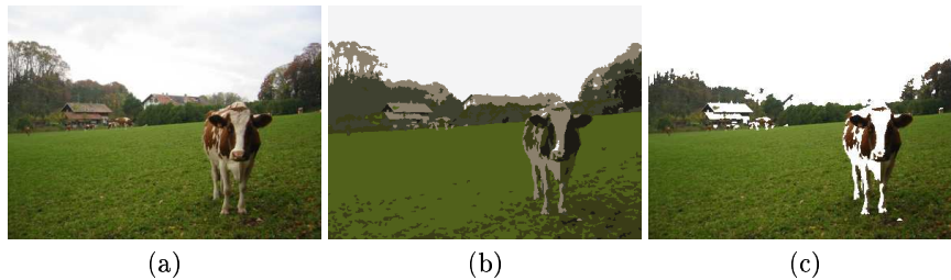
Fig. 1. The original image (a) is first segmented (b), and then we keep only the regions (c) the type of which has a large mutual information with the scene to predict. When indexing this image with respect to the countryside label, the sky and the buildings are considered as non-informative and are discarded.
