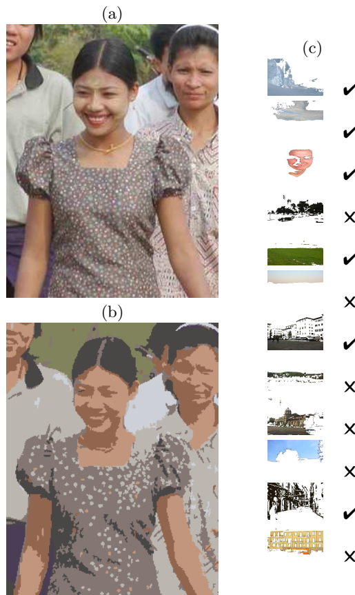
Figure 1: Feature extraction: the original image (a) is first segmented (b) then the corresponding boolean presence vector (c) is extracted by comparing the image regions to the typical ones obtained from the clustering of a training set.
